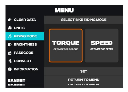
**Riding Mode:** You can switch to your preferred Riding Mode here (Torque, Speed). The default Riding Mode is 'Torque'.
