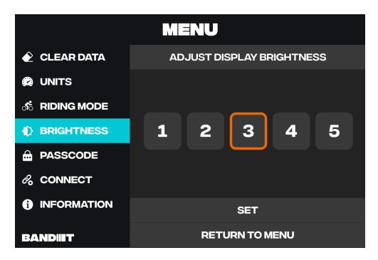
**Brightness:** Adjust your display's brightness level here. Brightness levels range from 1-5.
