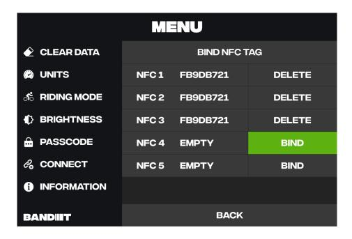
**Connect with NFC Card:** Connect your Bandit E-Bike with an NFC card to unlock your E-Bike more easily. You can have up to 5 NFC cards. Press 'Bind' To begin the pairing process.
